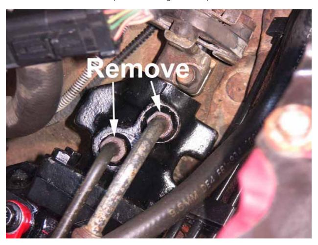
13.) Remove two of the three bolts on the driver's side frame that hold the box in place using 14MM socket. Loosen the remaining bolt but do not remove it until you are in place to support the steering box. If you are not prepared to support the box it can drop to the floor! Once the last bolt is removed the box will drop down and slide out from the bottom.
