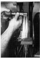
The spline end of the shaft is lightly sanded to make sure it is slightly under-sized. This will ensure that it fits the new bushings well. Now is the time to prep the shaft, not after you have installed the new roller, because you do not want anv debris in the new needle bearings.
