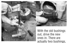
and they are driven in from the opposite ends of the box. Care is taken to drive the bushings in straight and square.
