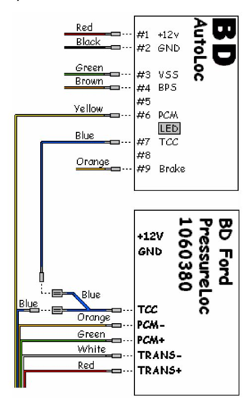
\*\*NOTE: YELLOW WIRE – Install a female spade connector and connect to the AUTOLOC Control Box PCM terminal. See next page for more details.
