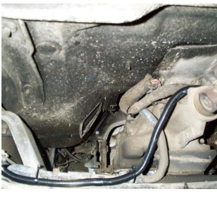
Run the PressureLoc wiring harness along the OEM wiring harness that runs over the transmission and along the rear cross-member and secure with it tie straps.
