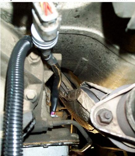
Remove the wiring connector plug from the transmission valve body controller.
