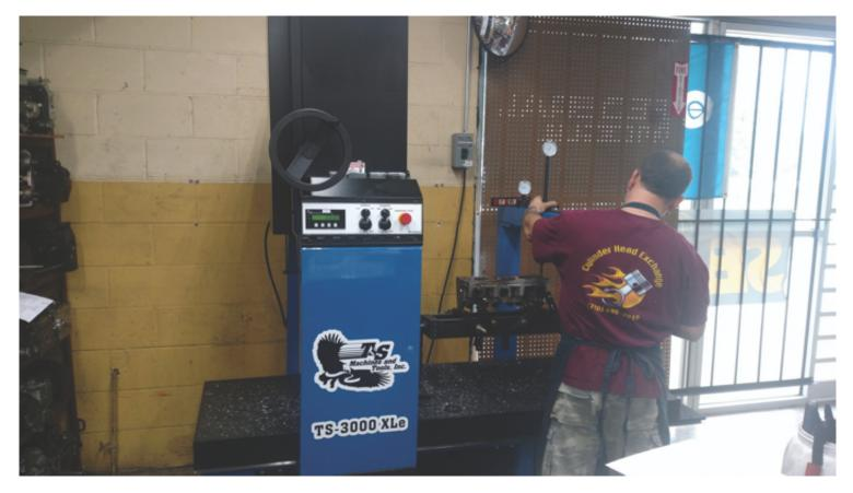
The final finish cut on any head should not exceed .001" A rough surfacing step followed by a final surfacing step will produce a better finish than trying to take off too much metal in a single pass.
