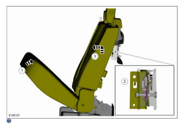
10. Pull the backrest release strap and fold the RH rear seat backrest down.
