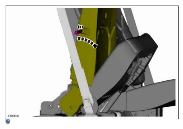
11. Release the clips and lower the headliner.
