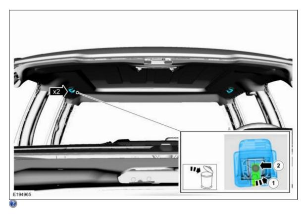
8. Disconnect the headliner wiring harness connectors, release the wiring harness retainer and position the wiring harness aside.
