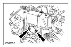
11. Remove the drive gear bolt and washer from the drive gear.
