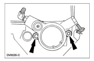
13. **NOTE:** If the high-pressure oil pump is to be replaced, remove the oil pressure regulator from the pump.
