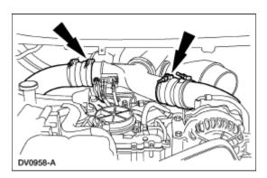
2. Label and disconnect the intake air temperature (IAT) sensor electrical connector, manifold absolute pressure (MAP) sensor electrical connector and the pressure hoses.
