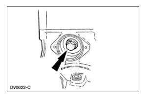
12. Remove the bolts and the high-pressure oil pump from the engine front cover. Remove and discard the gasket.
