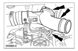
4. Remove and discard the compressor manifold O-ring seal.
