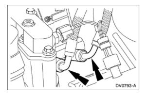
9. Disconnect the electrical connector from the oil pressure regulator.
