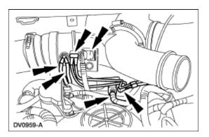
3. Loosen the clamps. Remove the compressor manifold.
