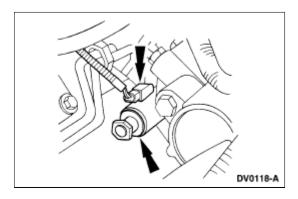
10. Remove the bolts and the cover from the engine front cover. Position the wiring harness aside.
