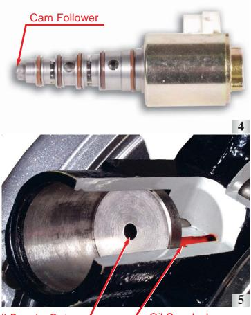
Oil Supply, Outer Side of Piston Oil Supply, Inner Side of Piston
