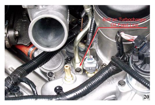
The snap-to-connect turbocharger oil feed line has been replaced with an o-ring sealed, bolt-on line. This was done to reduce leaks due to improper installation.
