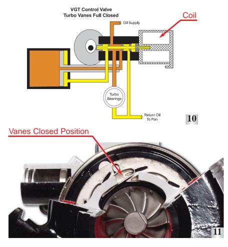
When the VGTCV is commanded to the full closed position, high duty cycle, oil from the oil supply line is directed through the actuator piston to the closed side of the piston.
