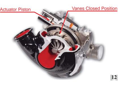
Closing the vanes also increases the back pressure in the exhaust manifold
