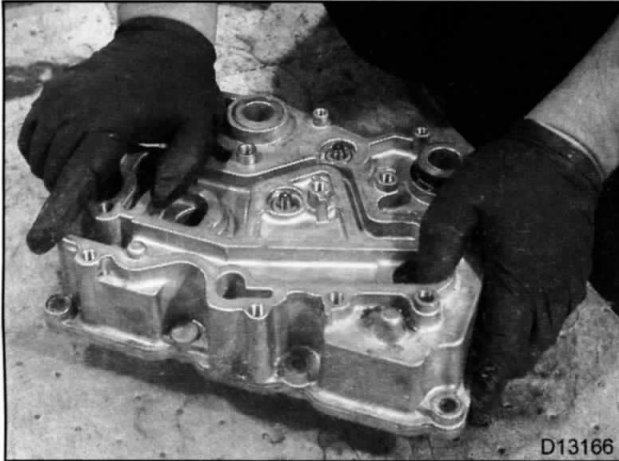
Figure 16 Installing oil cooler cover on to oil cooler
