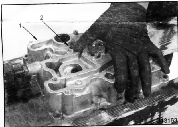
Figure 8 Removing threaded insert for oil cooler cover
