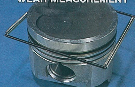
TOP RING GROOVE GAUGE PIN DIAMETER .115 in
