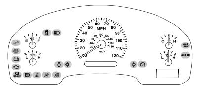
**Base with Tachometer instrument cluster**
