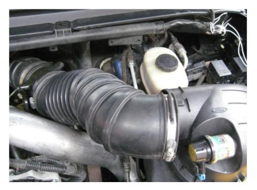
Then, loosen the 7/16" spring clamps for the intercooler boots, you do not need to remove them completely. Set the pipe aside. CAUTION: be careful when removing the intercooler pipe as the always hot feed to the alternator is near where you will be removing the pipe.
