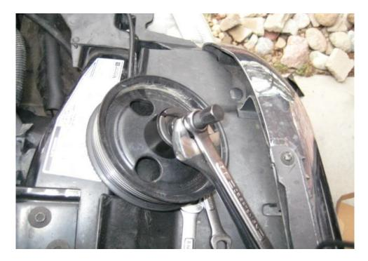
Now remove the three main bolts holding the pump to the bracket. These are 11/16" bolts and are pretty snug.
