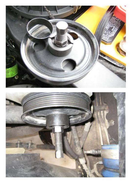
It takes quite a few cranks to get the pulley assembly off, but make sure that you always have your hand under the pulley as if it fell, the pulley could get damaged.
