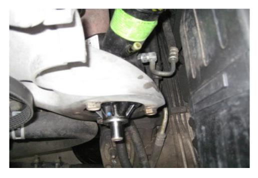
Once those three bolts are taken out, you can remove the lower clamp and hose from the old pump, and transfer it all to the new pump.
