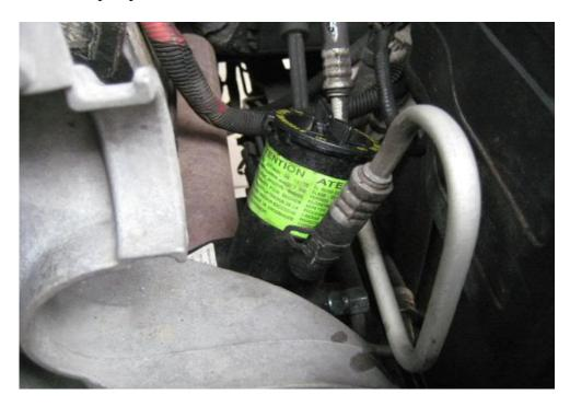
Now, remove the high pressure line from the pump, positioning your drain pan below pitman arm as fluid will start to drain out.
