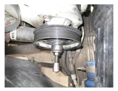
You can now reapply tension and route the belt how it was originally. Fill the reservoir on the pump with your Type F fluid. Start the truck and apply the brakes while steering lock to lock, paying attention not to hold the wheel at lock for too long. Do this a few times, then shut the truck off. Check the fluid level and top off accordingly.
