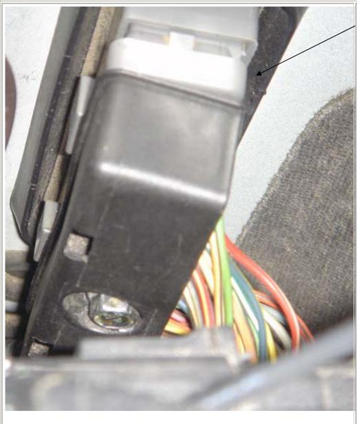
Using a mirror and flash light you can read the code located on the gray connector.
