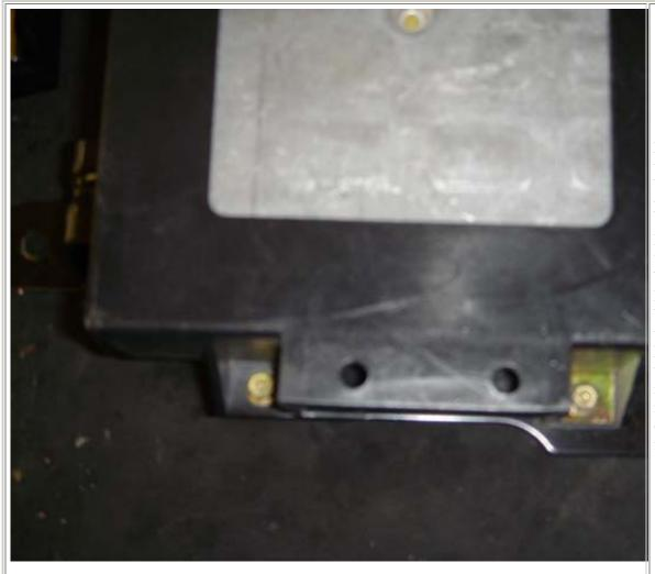
Locate the PCM inside truck. The PCM will be behind the emergency brake pedal, close to the drivers' side, kick panel area. Remove the top and bottom 7mm bolts holding the black plastic PCM housing. Remove the PCM and the black plastic housing from the drivers' compartment. Note how the PCM fits into the housing for reinstallation purposes. (In most cases there is an X on one side of the PCM, this X faces the fender.)
